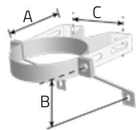
The wall band incorporates additional side support struts which can be located below or above the band. In either case the band is located under the female form at a joint between the components. Provides 50mm clearance from the wall. The maximum length which can be supported is 30 metres. Constructed from stainless steel.
