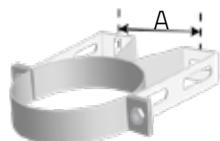
Provides 50mm clearance to structure
