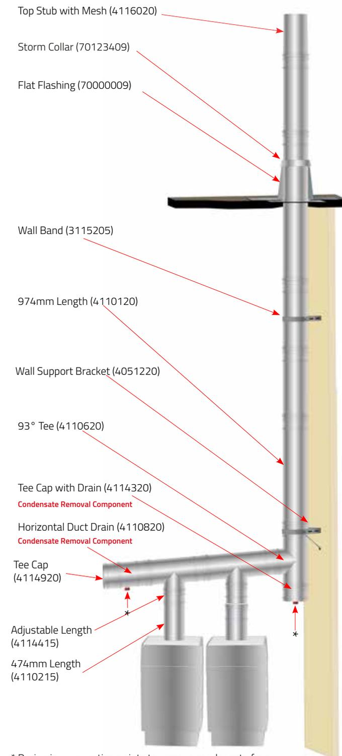
\* Drain pipe connection points to remove condensate from system to suitable drain.
