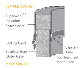
Sleeve joint with locking band for:
