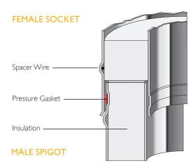
Sleeve joint with integral pressure gasket and locking band for:
