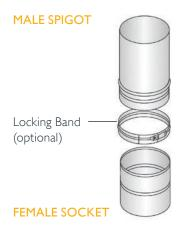
Sleeve joint with optional locking band for:
