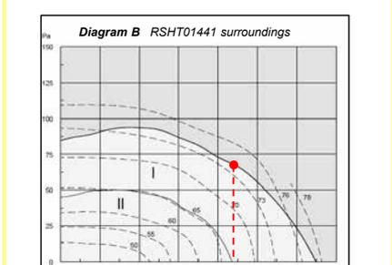
$K_{W1}$ : Correction factor for calculating sound output in the first octave band.
