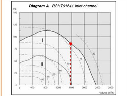
**Example:** For the values in **Table 4** and **Table 5** is read the factor ( $L_{WA3}$ ) in **Diagram B** at 2/3 of max. flow.
