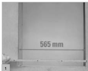
1 Clear installation width required 565mm.
