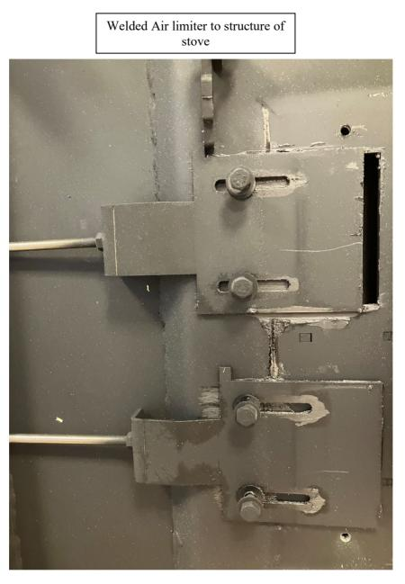
Tiverton Control Slide Plate leaves a 7 mm opening when fully closed.
