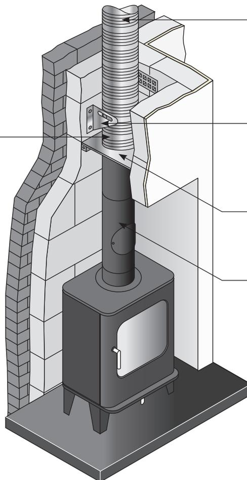
TecnoFlex Plus Liner Available in cut lengths or as packs containing the Top Clamp and Top Plate.
