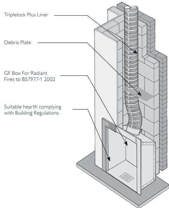
**When making a connection to a flue pipe in another product type, such as rigid stainless steel single or double wall or vitreous enamel, then the appropriate connector to/from flexible should be used. The connector should be suitably sealed to the appliance spigot ensuring a gas tight joint.**
